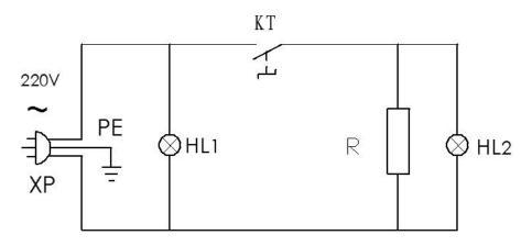
XP: Power Plug HL1: Power Indicator Light KT: Thermostat HL2: Heat Indicator Light R: Heating Element
