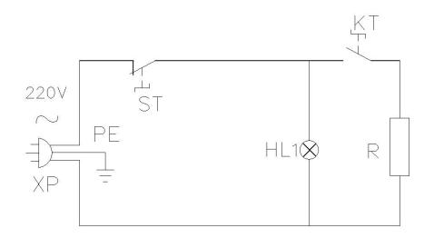
XP:Powe Cord HL1:Working Indicator Light R:Heating Element ST:Temperature Limiter KT:Temperature Controller
